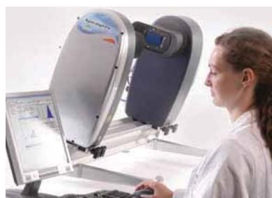
**2** Run the measurement by selecting the desired SOP from the menu system. This automatically configures the system and ensures everything is optimally set to deliver accurate results, including auto-alignment of the optical system. Synchronisation of external systems such as extractors, actuators and positioning systems is also supported.
