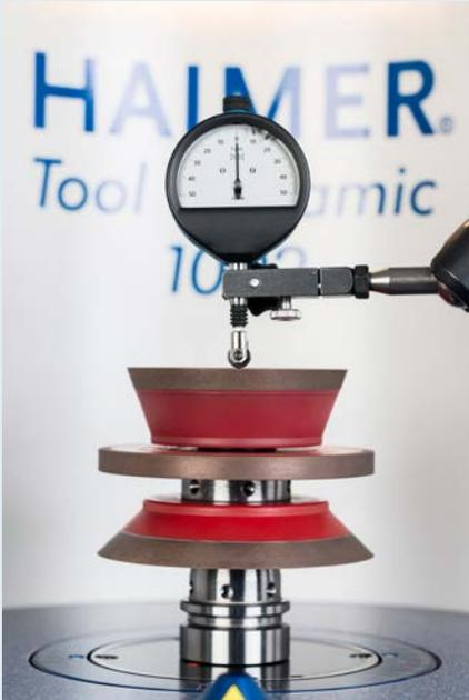
With the runout measuring device you can do an easy and reliable check of your grinding wheel's runout and axial runout. The runout measuring unit consists of: Measuring arm with tripod and fine indicator in 0.001 mm accuracy execution as well as a measuring roll.
