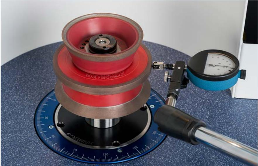
Measuring runout and axial runout as well as balancing without re-clamping!
