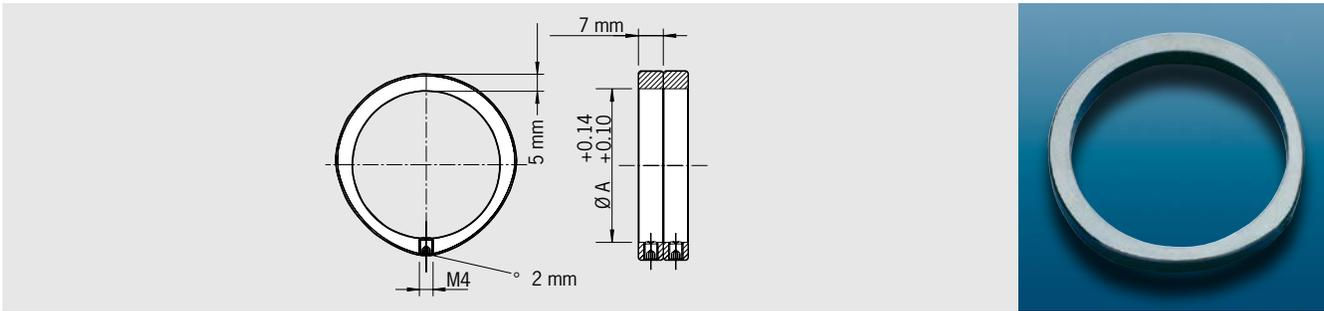
For fine-balancing of all tool holders with cylindrical outer diameters (diam. A)
