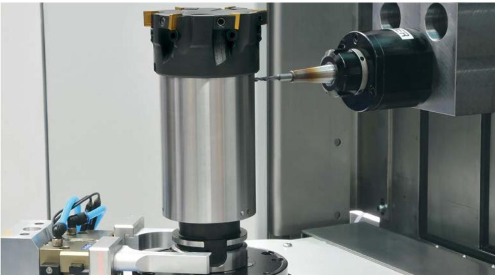
**Milling head, balancing in two planes**
