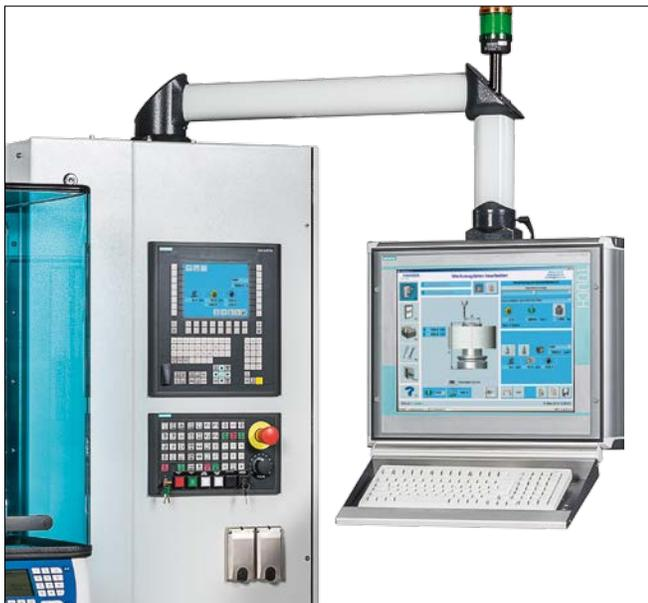
Integrated control and balancing software
