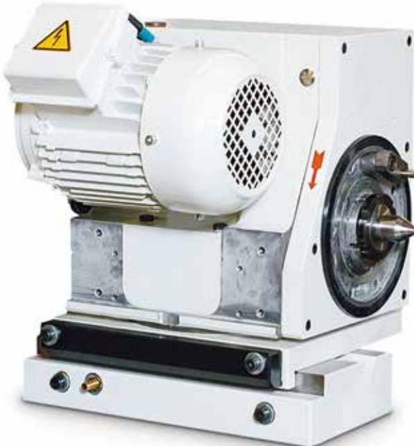
The swivelling workhead with hydrodynamic bearing makes it possible to grind between fixed centres as well as with rotating centres. The powerful workhead spindle, relieved from belt tension, rotates in a hydrodynamic multi-surface plain bearing. Roundness during live spindle grinding is 0.0003 mm (0.000,012"), with the option of 0.0001 mm (0.000,004") available. The workhead is driven by a stepped AC motor.
