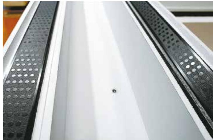
① Machine base with longitudinal and cross guides
