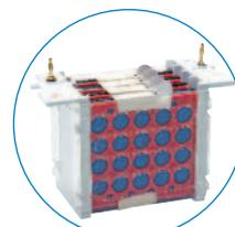
**High Intensity Electroblotting Module** – with 2 blotting cassettes and Platinum plate electrodes, the high intensity blotting module allows fast transfer of proteins to membranes with excellent time savings.
