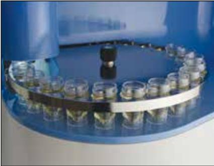
An external load-and-go sample tray allows for continuous loading of cell culture samples for the most flexible and efficient sample throughput.
