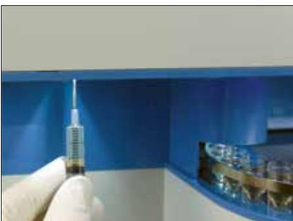
Individual samples also can be analyzed directly from syringes or cups. Batch sampling via the 96-well plate and/or external "load-and-go" sample tray runs can be interrupted at any time to run critical gas syringe samples.
