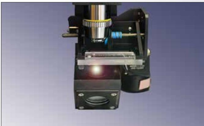
FLEX2 high resolution optics count cells as small as 4 microns
