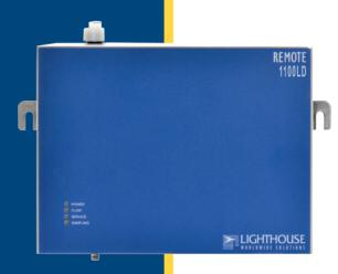
SING state-of-the-art long life laser diode technology, the Lighthouse Remote 1104LD is an industry first laser diode based remote particle counter with a sensitivity of 0.10 µm at a high flow rate of 1.0 CFM (28.3 LPM) that uses an optics and photodiode system designed to reduce or eliminate the temerature issues associated with high power laser diode sensors.
