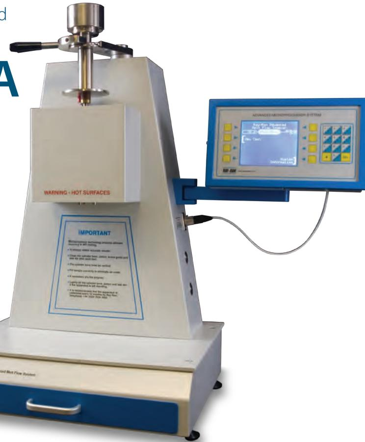
each slice during the test. For quality control purposes the 6MPCA microprocessor can be set with High and Low limits which are clearly defined when the results are downloaded to a PC showing the user instantly if the material is a pass or fail.
