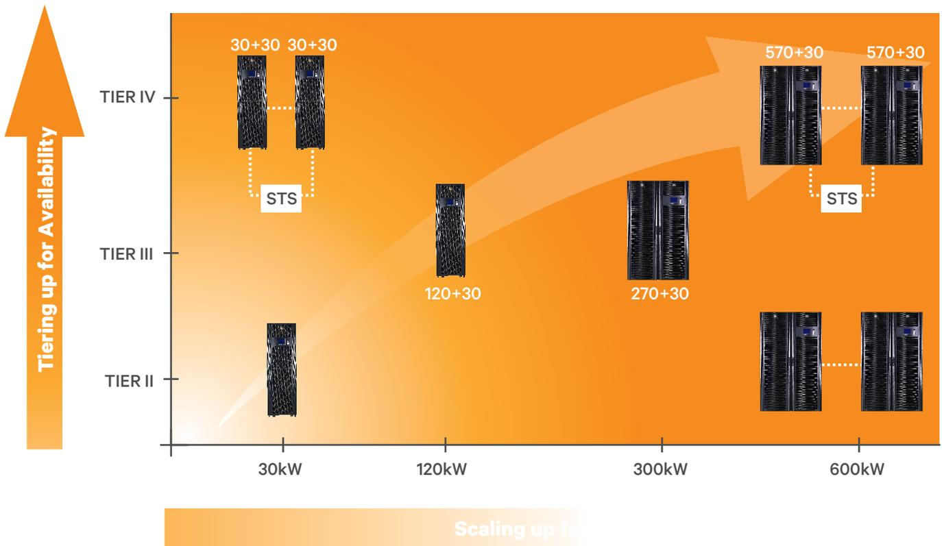
The Liebert® APM™ system can be utilized with either single or dual power inputs. The dual power features allows you to take advantage of a secondary power source. In addition, up to 4 racks can be paralleled to achieve increased redundancy for more power and 2 sets of racks can be deployed in a Dual Bus architecture.
