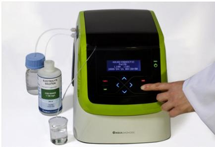
COD results in just 15 minutes, with no use of dichromate. PeCOD® is breaking the barriers to traditional COD analysis methods.
