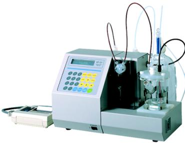
KF-21 volumetric moisture meter is both compact and portable ideal for routine moisture analysis in the field or laboratory and a reagent dispenser comes as standard. CA-21 Coulometric/KF-21 Volumetric Karl Fischer Moisture Meter complies with the following standards:
