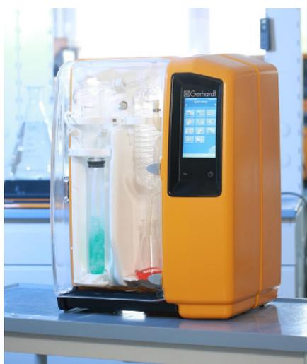
VAPODEST watersteam rapid distillation systems by Gerhardt are used worldwide, e.g. for the determination of nitrate, nitrite, ammonium, Kjeldahl digestion solutions, volatile acids, sulphur dioxide,
