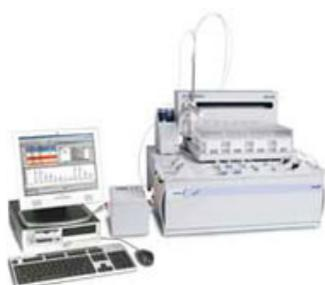
For 20 years, Lachat Instruments has led the world in productivity for automated ion analysis based on flow injection analysis (FIA) technology. The simplicity and ruggedness of FIA, the outstanding accuracy, precision, low detection limits and dynamic ranges of our guaranteed QuickChem methods and our unique Data Quality Management closed-loop
