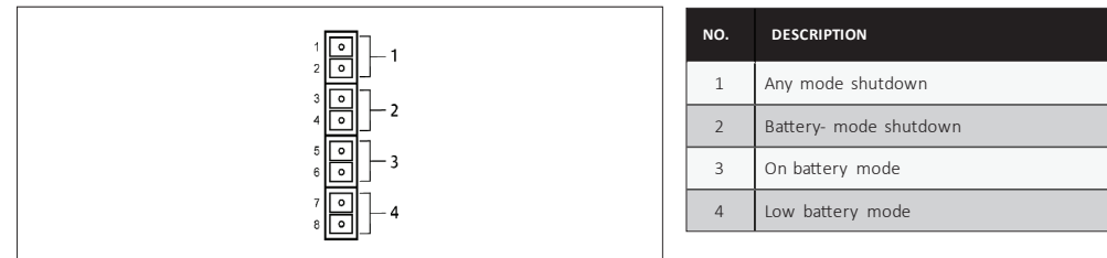
Figure 2.1 Terminal-block communication pin layout
